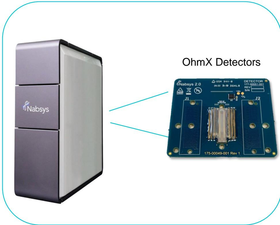
Labeled linear DNA flows through nanochannel detectors allowing for data capture
