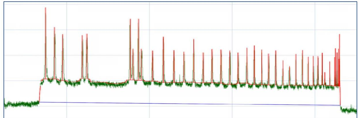
Real-time signal processing registers a voltage change over time for every tag on every DNA molecule
